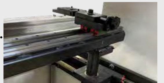
Arka Dayamada Opsiyonel Motorlu R Eksen Optional Motorized R Axis on Backgauge
