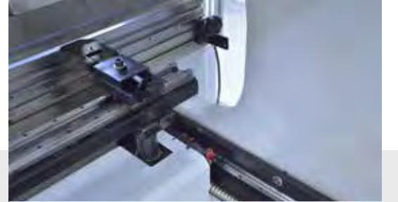
Motorlu Vidalı Mil Arka Dayama Motorized Backgauge with Ballscrew
