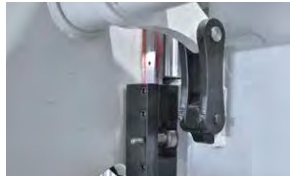
Hassas Büküm sağlayan dengeleme kolu Torsion bar enabling sensitive bending
